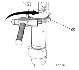
15. Install coupling (125) around pump rod.
